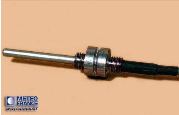
It is a device measuring temperature by the reversible change of the electrical resistance of a metal wire.
