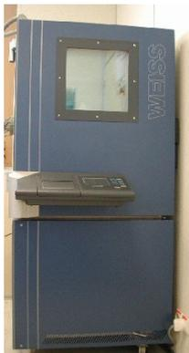
Used when it is impossible to immerse the sensors in a fluid (thermohygrometer...), the calibration is made in the air.
