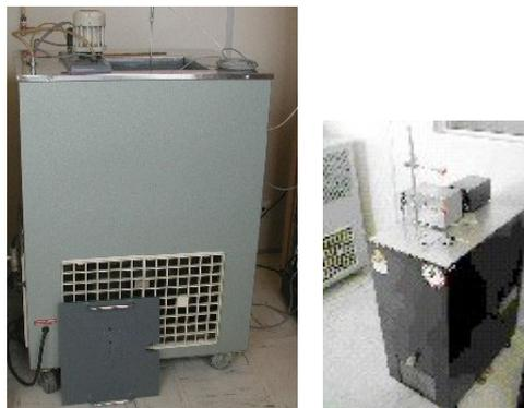
*Photo 1: Baths for temperature calibration*
