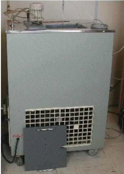
To obtain the best stability, both special fluid and thermal block of equalization are used in a bath. Alcohol, water or oil are used according to the wanted range of temperature.
