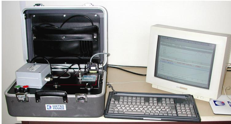
*Photo 3: In situ pressure calibration system*
